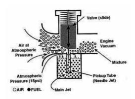
Both the CV and conventional slide carburettors, like Amals, are classified as variable venturi carbs. The slide on a conventional carburettor is directly connected to the throttle cable. Twist the throttle grip and the slide is raised in the venturi.
