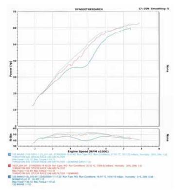
line from the Bonneville with the top red line. No mid range hole! The result is that between 50mph and 80mph the Thruxton is a joy to ride. There is always ample power to overtake without chasing the torque peak, it is there, all 53 ft lbs of it, from 3500 to 6000 rpm
